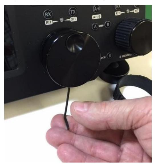
Once the set screw is loosened, slide the knob off the encoder shaft by gently pulling the knob forward.
