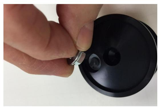
Below is an image showing the counterweight properly seated in the finger dimple recess hole.
