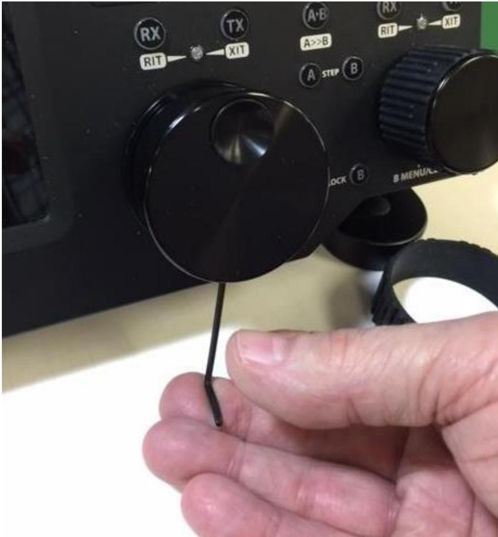
Once the set screw is loosened, slide the knob off the encoder shaft by gently pulling the knob forward.
